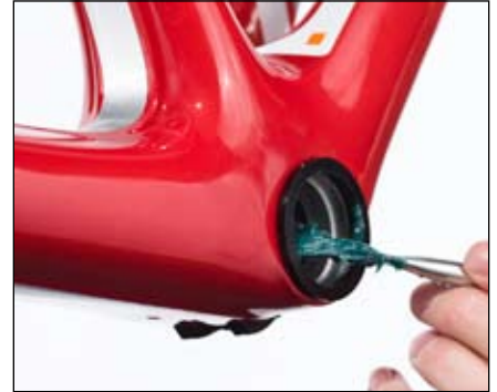
Figure 43. Greasing the bearing cups
